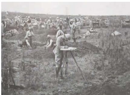
A French soldier using a plain table to survey an artillery battery position, c1917
